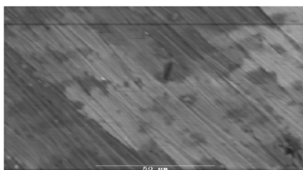
图1 未添加 DBDS 油样中铜片 48h 后的 SEM 表面形貌 (500 倍) Fig1 the SEM surface morphology of copper sheet without the DBDS in oil sample 48h(500 times)
